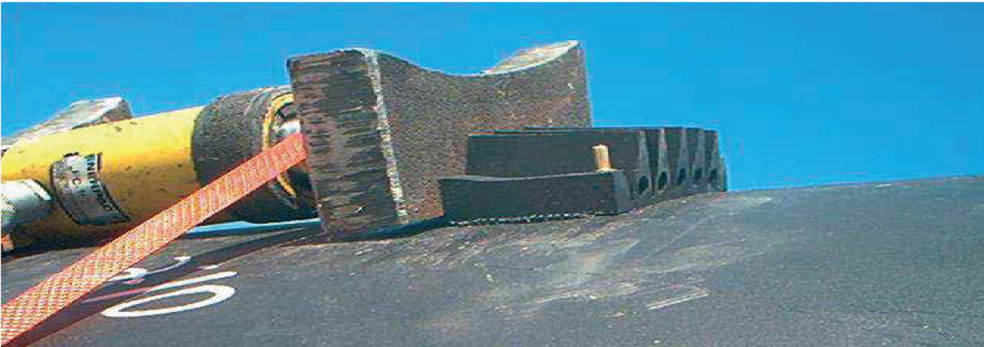
FIG. 1 Electrofusion Flex Restraints Tested to 10,000 lbs Axial Force
